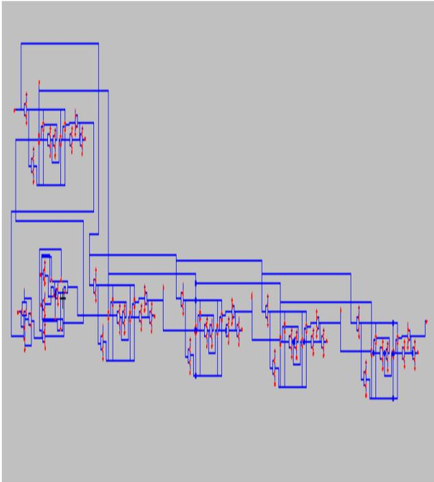
Fig. 10 Schematic of sequential 4-bit adder using the proposed full adder cell
